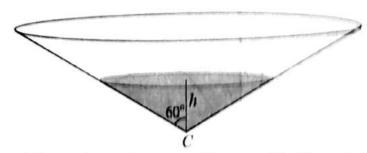
A tank containing water is in the form of a cone with vertex C. The axis is vertical and the semivertical angle is  $60^{\circ}$ , as shown in the diagram. At time t = 0, the tank is full and the depth of  $\frac{1}{1000}$ is H. At this instant, a tap at C is opened and water begins to flow out. The volume of water in the tank decreases at a rate proportional to  $\sqrt{h}$ , where h is the depth of water at time t. The tank becomes empty when t = 60.
